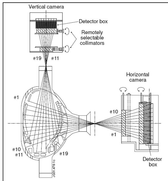
Figure 1. Schematic view of the JET neutron emission profile monitor showing the lines of sight.
