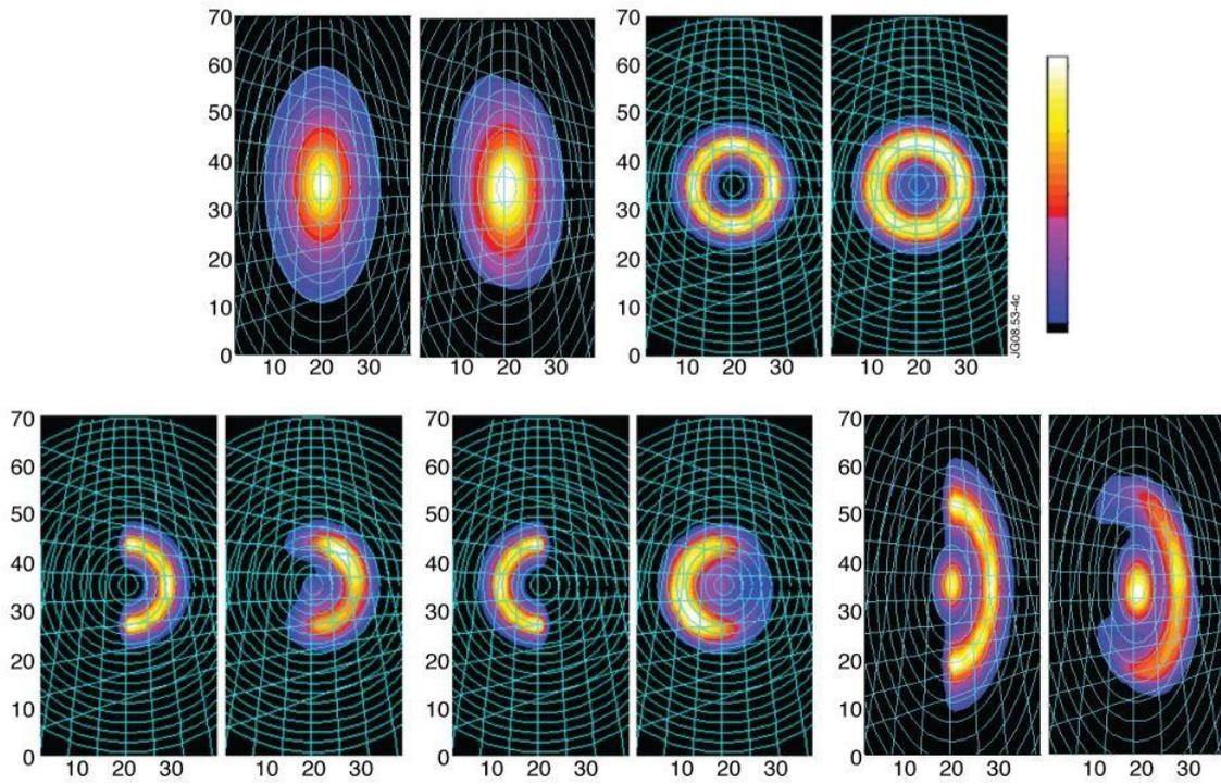
Figure 2 - The test phantoms and their ML reconstruction: peak (top-left), hollow (top-right), “banana” (bottom-left), symmetrically reversed “banana” (bottom-middle) and banana plus peak (bottom-right). In each case the phantom is presented in the left side of the illustration and the reconstruction in the right one.
