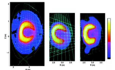
'Peak plus banana' profile distribution recorded just after the T-puff, when tritons partly penetrated into the plasma core from the periphery—shot 61132 at 62.67 s
