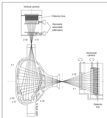
Schematic view of the JET neutron emission profile monitor
